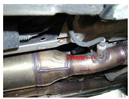
If you have a Peake R5/FCX scan tool (<a href="http://www.peakeresearch.com/code\_tool.shtml">http://www.peakeresearch.com/code\_tool.shtml</a>), now would be a good time to reset the check engine light. The Peake was also used to initially diagnose the problem and identify the passenger side Pre-Cat O2 Sensor as the failed component.
